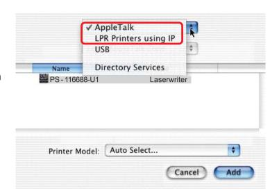
AppleTalk protocol: After selecting AppleTalk the Port Name of the Print Server will be displayed. The Port Name shown here is an example only.
